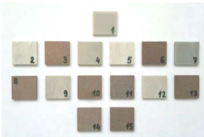
Fig. 1. Samples for abrasive wear resistance test: 1 – unmodified POM, 2-7 – two-component composites POM, 8-9 – three-component composites POM, 14-15 – four-component composites POM
