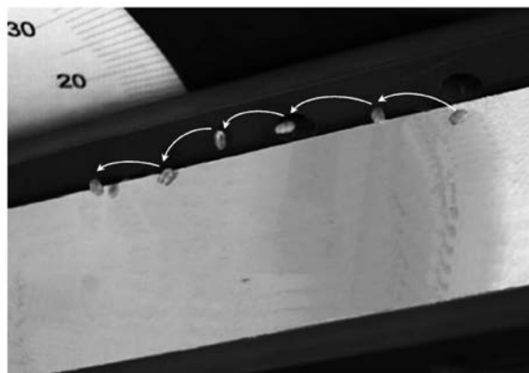
Fig. 6. Visualization of the trajectory traveled by a kernel on an inclined plate during measurements of movement parameters
